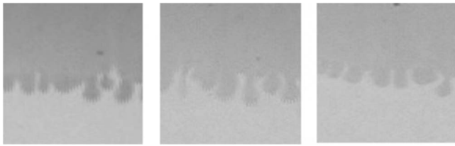
FIG. 4. Fingering patterns observed for various initial interface thicknesses (from left, to right: \delta \approx 8e, 15e, 19e ), at front locations l_f \approx 25e, 41e, 57e , respectively.
