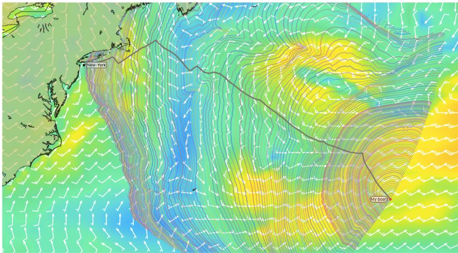
Figure 4: Result of a simulation by the method of isochrones using the software qtVlm for a navigation starting from an initial position in the middle of the Atlantic up to New-York. Background colors and vectors correspond to the initial weather prediction. The curves are the computed isochrones. The optimal trajectory is the thick line that crosses the isochrones. This trajectory presents a number of cusps that correspond to upwind or downwind tacks.
