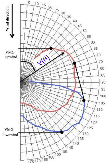
Figure 2: Speed diagram of a sailing boat for a given wind intensity and sea state. This polar curve represents the best velocity  $V(\theta)$  of the boat when sailing at angle  $\theta$  with the direction of the incoming true wind. The red and blue curves correspond to different front sails, and the three black lines correspond to the convex envelope of the speed diagram.
