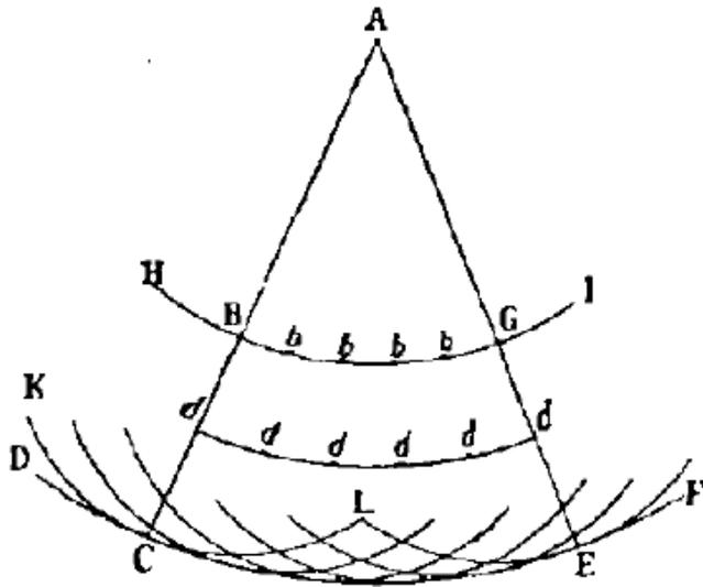
Figure 5: Drawing of Christian Huygens in his "Traité de la lumière" (1690). Each point of a wavefront at time  $t$  is a source of circular waves. The envelop of all the circular waves gives the new wavefront at time  $t + \Delta t$ .
