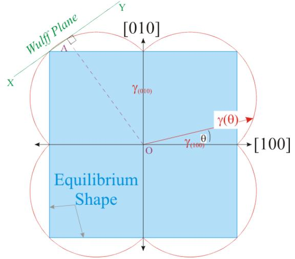
Figure 3: Wulff construction (from Wikipedia) giving the equilibrium shape of a crystal as the inner envelope of the polar surface energy  $\gamma(\theta)$ .
