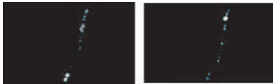
Fig. 2. Few cavitating bubbles aligned along a vertical filament, in stroboscopic lighting (exposure time 20 \mu s), vertical field of view is 6.8 cm. From one picture to the other one, vapor bubbles are different but clearly cavitate from the same region.
