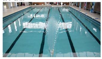
FIG. 2. (Color online) Wake patterns in the swimming pool experiments, for a cylinder of diameter D=16 mm (Bond number  $Bo_D=1.0$ ), at velocity U=0.63 and 2.5 m s<sup>-1</sup>. The wake angle is determined from the intersection (shown by the vertical arrow) of the dashed line, going through the waves of maximum amplitude, to the back edge of the pool.
