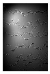
Non-invasive optical techniques will be used to measure the liquid film thickness (synthetic Schlieren method, Chromatic Confocal Imaging method), the gas velocity (PIV) and the temperature field in the liquid phase (Liquid Cristal thermometry).
