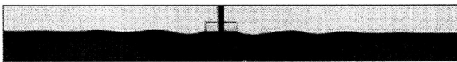
FIG. 2. Snapshot of the waves generated at the top of a fluidized bed. The volume fraction is \Phi \approx 0.37 , the suspending fluid is water, and the beads are 125 \mu\text{m} in diameter. (Window width: 22 cm of the 50 cm wide Hele-Shaw cell.)
