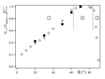
FIG. 4. Compared variations with the tilt angle  $\theta$  of the experimental normalized stationary front velocity  $V_{f^{\infty}}/V_{\text{plateau}}$  ( $\diamond$ ) and of  $\sqrt{C_{f^{\infty}}}$  ( $\blacksquare$ ) computed from concentrations measured experimentally (the values of  $\mu$  and At are the same as in Figs. 2 and 3).
