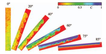
FIG. 2. (Color) Images of the normalized relative fraction of light fluid obtained at different tilt angles  $\theta$ =0, 20°, 40°, 60°, 75°, and 85° (field of view=20×300 mm). The color code for the normalized fraction is shown at the top right of the figure. The magnification of the images of the tube is higher perpendicular compared to parallel to the tube axis.
