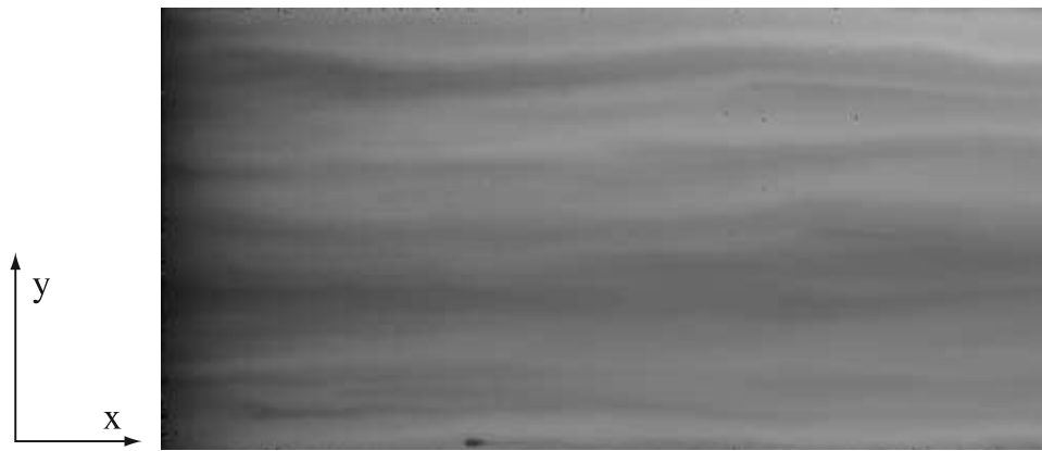
Figure 6. Gray scale map of the normalized local transit time \overline{t(x,y)U/x} . Flow is from left to right. Dark (light) regions correspond to locations where \overline{t(x,y)U/x} < 1 ( \overline{t(x,y)U/x} > 1 ). Mean flow velocity U = 0.014 mm/s ( Pe = 150 , polymer concentration 1000 ppm). The map covers the total area of the model fracture (size 85 \times 171 mm).
