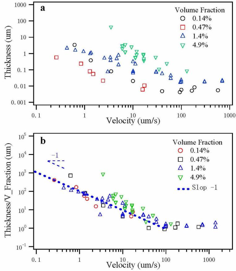
Figure 3: a. Mean thickness as a function of velocity for various particle volume fraction. b. Mean thickness over particle volume fraction ratio as a function of velocity.
