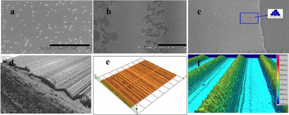
Figure 2: Scanning electron microscopy images of the deposition a.  $V=572\mu\text{m/s}$ ,  $\phi=0.47\%$  b.  $V=29.4\mu\text{m/s}$ ,  $\phi=0.47\%$  c. Zoom-in of image b. for sketch of typical closed-packed particle aggregation. Optical profile images of deposition pattern d.  $V=1\mu\text{m/s}$ ,  $\phi=1.4\%$  e.  $V=4.5\mu\text{m/s}$ ,  $\phi=0.47\%$  f.  $V=5\mu\text{m/s}$ ,  $\phi=4.9\%$ .
