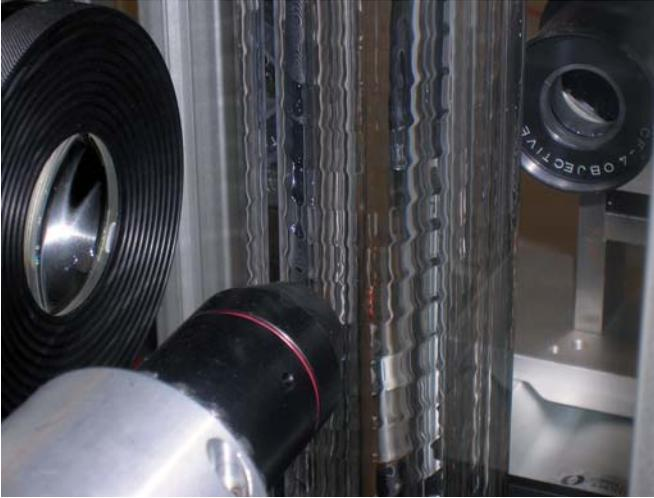
Figure 4.6: Photograph of 2-dimensional wave fronts in the optical test setup:  $Re=12.9$ ,  $Ka=509.5$ ,  $f=24$  Hz.
