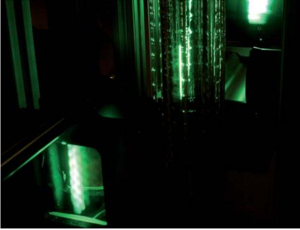
Figure 4.33: Photograph of the PIV laser light sheet illuminating the wavy liquid film in the optical test setup.
