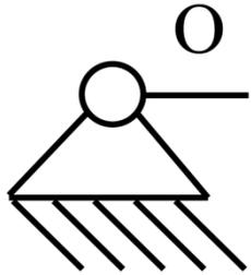
$$\begin{cases} \underline{R}(s = 0) = -\underline{R}_O \\ \underline{M}(s = 0) = \underline{0} \\ \underline{\Omega}(s = 0) = \underline{?} \\ \underline{U}(s = 0) = \underline{0} \end{cases}$$
