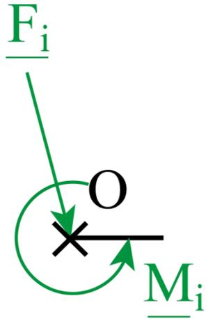
$$\begin{cases} \underline{R}(s = 0) = -\underline{F}_i \\ \underline{M}(s = 0) = -\underline{M}_i \\ \underline{\Omega}(s = 0) = \underline{?} \\ \underline{U}(s = 0) = \underline{?} \end{cases}$$
