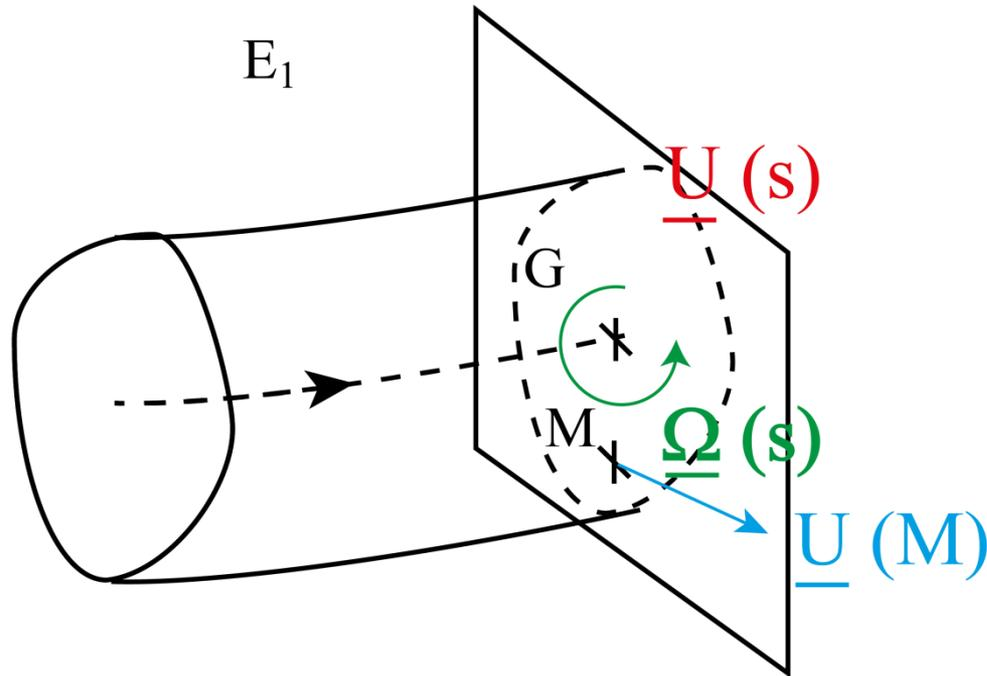
$$\underline{U}(M) = \underline{U}(s) + \underline{\Omega}(s) \wedge \underline{GM}$$
