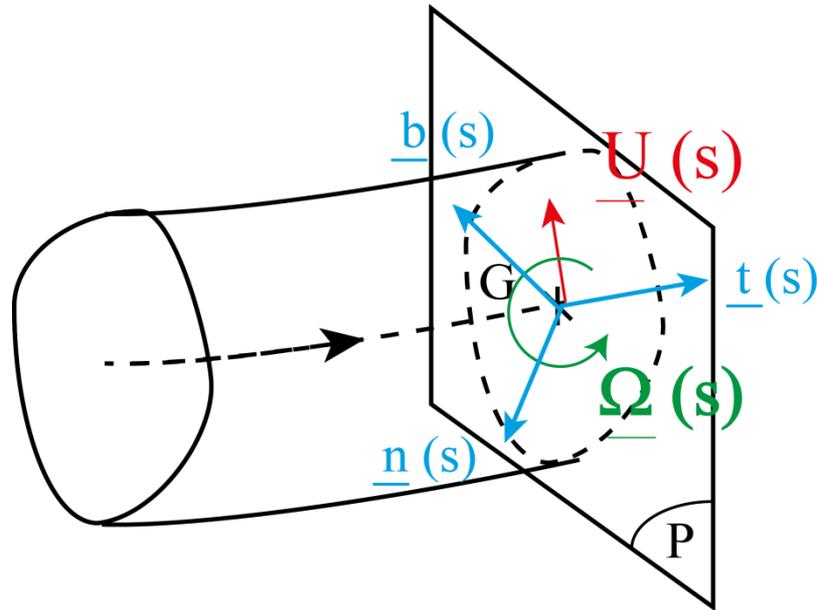
$$\underline{\Omega}(s) = \omega_t \underline{t} + \omega_n \underline{n} + \omega_b \underline{b}$$
