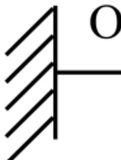
$$\left\{ \begin{array}{l} \underline{R}(s = 0) = -\underline{R}_O \\ \underline{M}(s = 0) = -\underline{M}_O \\ \underline{\Omega}(s = 0) = \underline{0} \\ \underline{U}(s = 0) = \underline{0} \end{array} \right.$$
