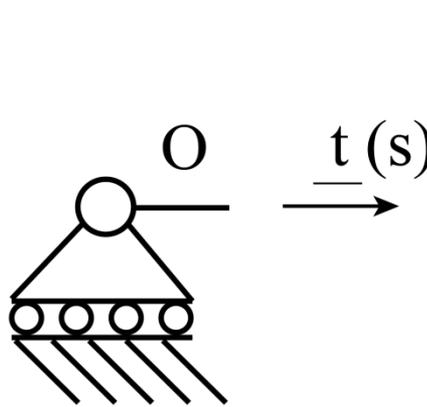
$$\left\{ \begin{array}{l} \underline{R}(s = 0) \cdot \underline{t}(s = 0) = 0 \\ \underline{M}(s = 0) = \underline{0} \end{array} \right.$$
