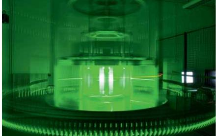
A Liquid Foucault Pendulum observed the Coriolis force using the Giroflow rotating platform, at the center of which lies a water-filled sphere.
