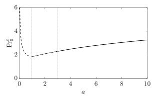
FIG. 7. Critical Froude number  $Fr_0^c = \sqrt{H_0/h_0^c}$  at which the maximum wave amplitude is reached for the collapse of a granular column, as a function of the initial aspect ratio a. The line corresponds to Eqs. (A1) for the three domains separated by the two vertical dotted lines at a = 0.93 and a = 3.
