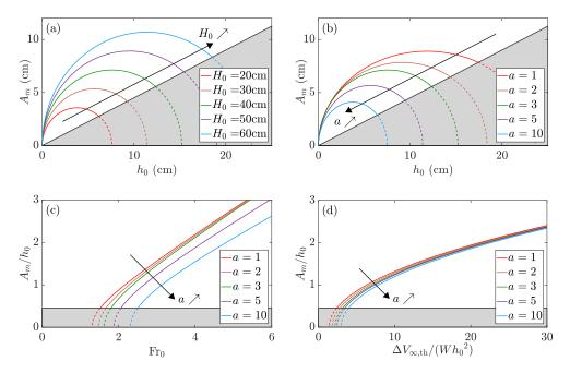
FIG. 5. (a), (b) Maximum wave amplitude  $A_m$ , given by Eq. (5), as a function of the water depth  $h_0$ , for (a) different initial height  $H_0$  with the same aspect ratio a=3 and (b) different a with  $H_0=40$  cm. (c), (d)  $A_m/h_0$  as a function of (c) Fr<sub>0</sub> as given by Eq. (6) and (d)  $\Delta V_{\infty,\text{th}}/(W h_0^2)$  as given by Eq. (7), for  $H_0=40$  cm and different a. Shaded areas are the same as in Fig. 2.
