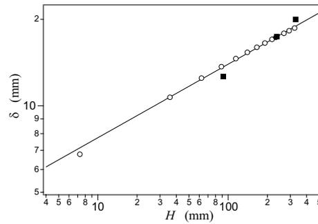
**Fig. 3.** Penetration depth  $\delta$  versus the total drop distance  $H$ . (■) Experimental measurements; (○) numerical values; (—) the adjustment is a power law of the form  $\delta = AH^\lambda$  with  $\lambda \simeq 1/4$  and  $A \simeq 4.3$  S.I..
