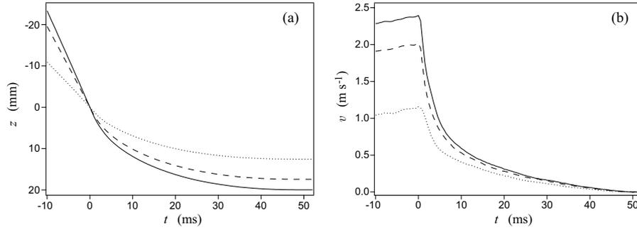
**Fig. 1.** (a) Position  $z$  and (b) velocity  $v$  of the projectile versus time for three different drop heights: (· ·)  $h=75$  mm, (– –)  $h=215$  mm, (—)  $h=305$  mm.
