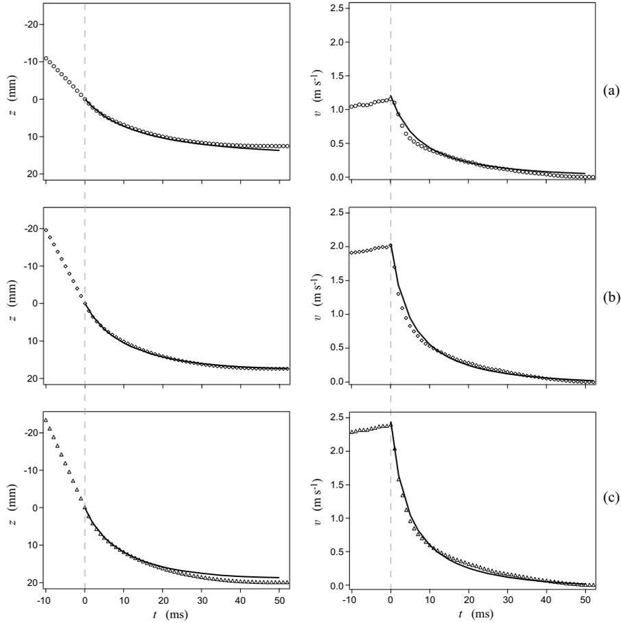
**Fig. 2.** Position  $z$  and velocity  $v$  of the projectile as a function of time for (a)  $h=75$  mm, (b)  $h=215$  mm, (c)  $h=305$  mm. (—) Best fit of experimental data with numerical values  $\alpha_f=6 \text{ kg s}^{-2}$ ,  $\alpha_c=0.7 \text{ kg s}^{-1}$  and  $\alpha_v=0.58 \text{ kg m}^{-1}$ . (- -) Time at which the impact occurs.
